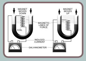
moving a magnet relative to the coil can produce a voltage as shown on the galvanometer. This voltage can then drive electrical current through standard power lines for use in homes or businesses. The illustration below shows the parts of a wind turbine.
